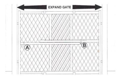
1. Facing locking mechanism, move security loop A to left of notched bar. Pivot retaining loop B to point straight up. Expand gate by hand for a snug fit in doorway or hallway from 27" to 41". Make sure all four rubber bumpers engage inside of door jam or firm wall surfaces.
