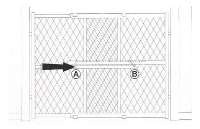
4. Slide security loop A onto notched bar and drop into first notch. Check to be sure gate is secure by grasping top and attempt to move toward and away from you. If gate is not secure, release gate and repeat steps 3 and 4 moving loop B to left one notch at a time until secure.
