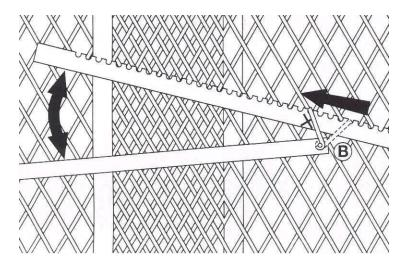
3. Raise notched bar at left (free) end, and position top of loop B into marked notch. Push down on left end of notched bar so gate expands into position.
