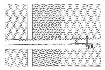
2. Holding loop B straight up, count four notches to left (toward free end) and make a distinctive pencil mark on notched bar. Repeat steps 1 and 2 each time the gate is used at a different location.
